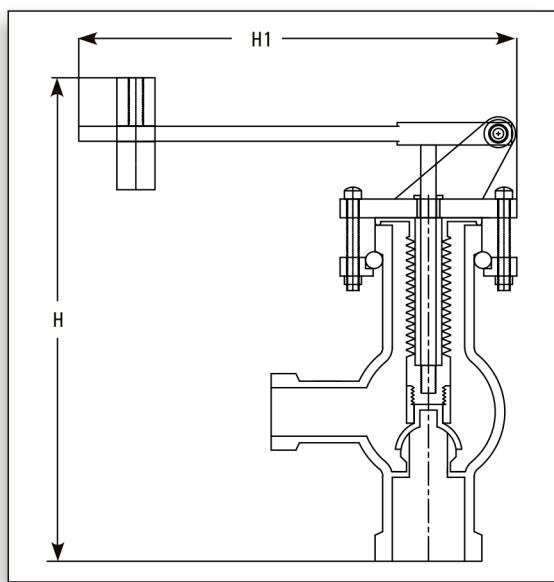
The pressure relief valve (WPRV) is a valve used to control or limit the pressure in a system or vessel which can build up by a process upset, instrument or equipment failure, or fire.
